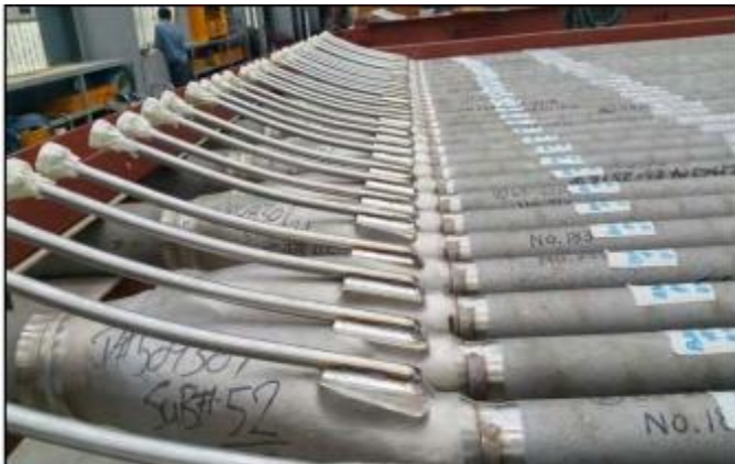
TETRA FITTING WELDING
