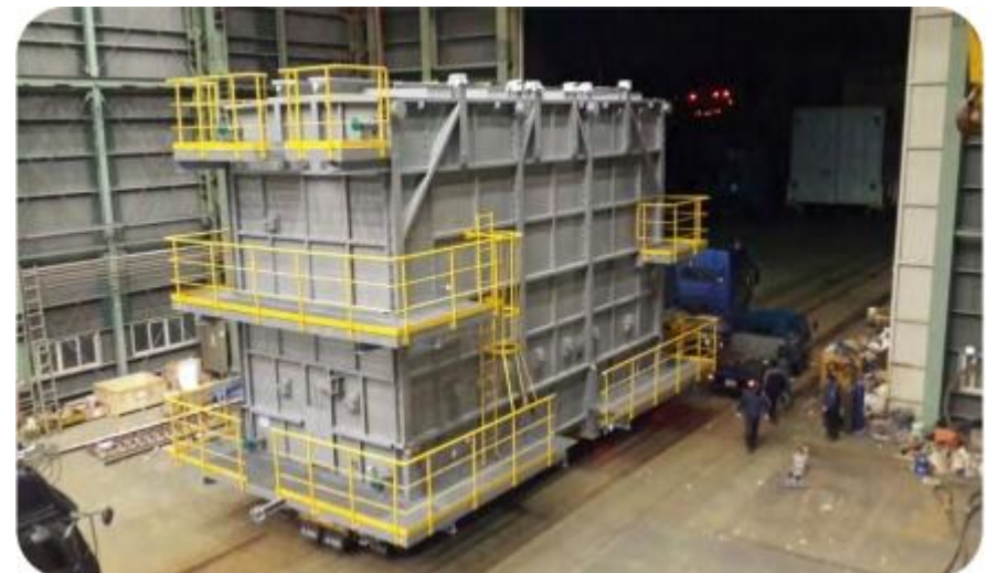
RADIANT MODULE TRANSPORTATION
