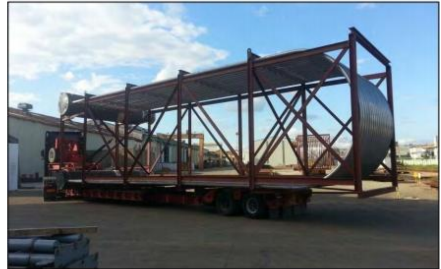
RADIANT ABOR COIL TRANSPORTATION
