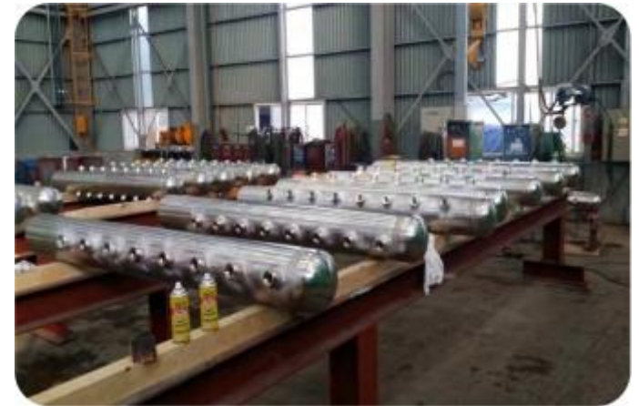
OUTLET HEADER WELDING
